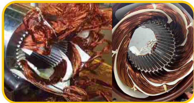
1 : Typical random winding being inserted in stator slots.
