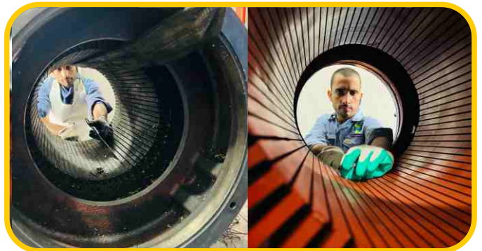
Picture 2 : A special tool is used to insert the stator slot wedges from the side of the core.
